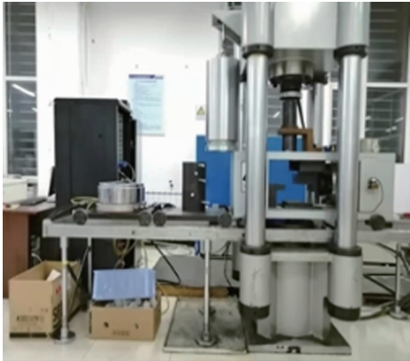
图 2 TAW-2000 电液伺服岩石三轴试验机 Fig. 2 TAW-2000 electro-hydraulic servo triaxial testing machine
