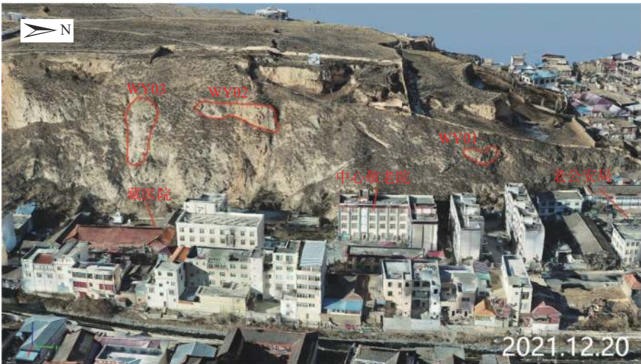
图 4 北侧危岩带分布示意图 Fig. 4 Schematic diagram of the distribution of hazardous rock zone on the north side
