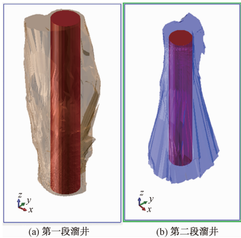
图 4 溜井垮塌前三维模型与实测溜井垮塌模型复合图 Fig. 4 The model composite diagram of measured ore-pass model and 3D model before the collapse
