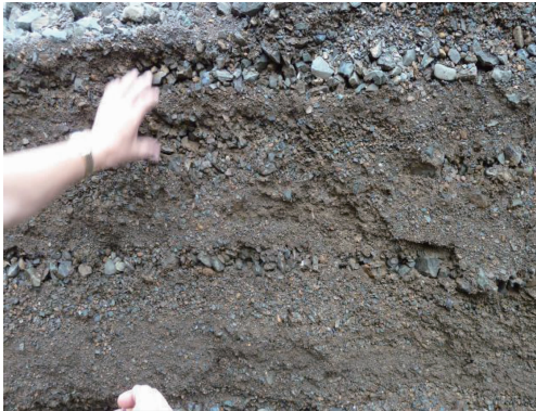
图12 泥石流堆积层 Fig.12 Accumulation horizon of debris flow
