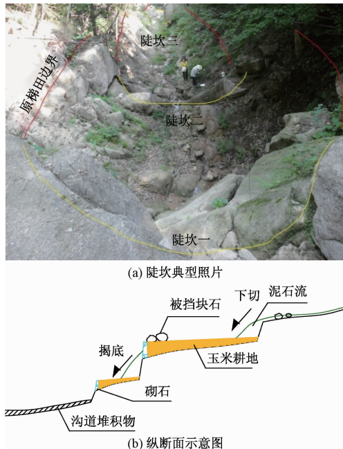
图 3 上疙瘩沟陡坎典型照片和纵断面示意图 Fig. 3 Typical picture and schematic diagram of the scarp in Shanggeda gully
